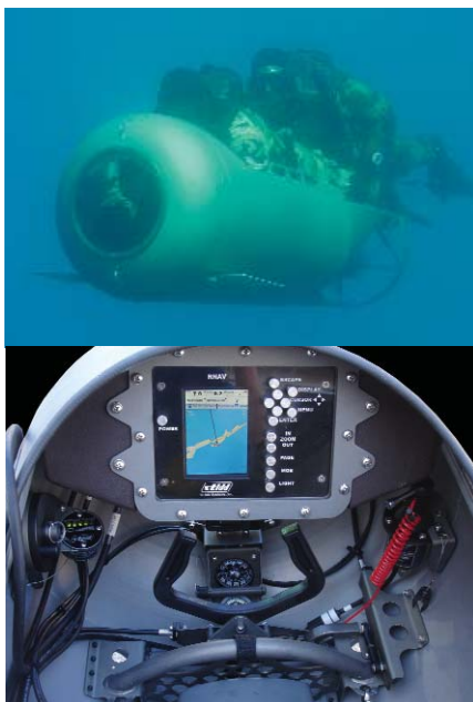
Top: STIDD Diver Propulsion Device (DPD). Below: RNAV is an advanced electronic navigation system purpose built for the STIDD DPD. STIDD photos.
