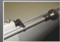
The RNAV mast easily folds-down to stow and lock when not in use.
