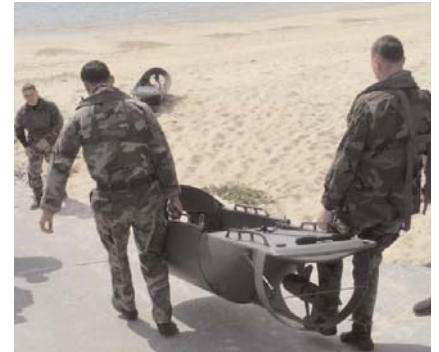
The STIDD DPD, weighing in at 159 pounds complete, is easily carried by two persons.
