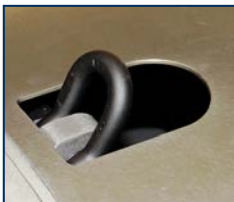
Bow tow-eye for quick link to DPD
