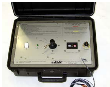
DPD Thruster Bench Test Power Supply is included with DPD Long Term Maintenance Special Tools.
