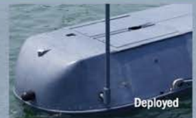
The MRCC is the only submersible that allows divers and equipment to travel on the surface over long distances to the point of submerging, minimizing divers immersion time in water.
