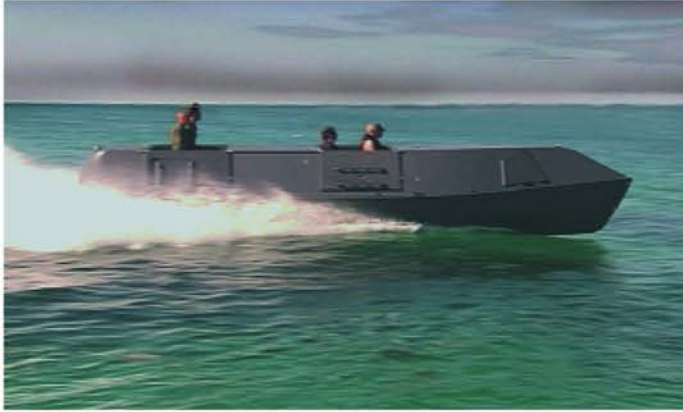
MRCC operates in surface planing mode with diesel/waterjet propulsion
