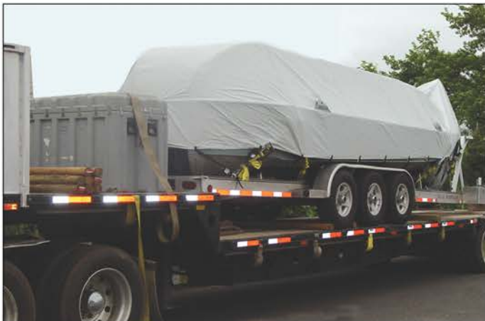
STIDD DPD in reusable shipping container and MRCC shoaw loaded for long distance land transport complete with MRCC trailer and transportation cover.
