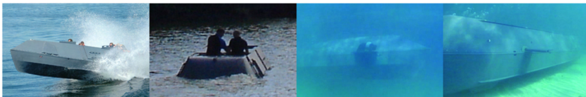
STIDD 32.5 MRCC Multi-Role Combatant Craft offers a fast surface boat, reduced semi-submerged observability and submerged propulsion in one package.
