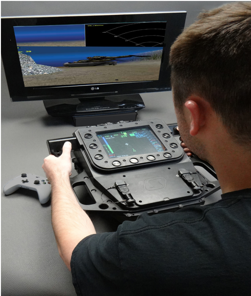
"Operator using RNAV2 Training Simulator System to mimic training dive profile"
