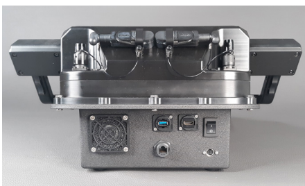
RNAV2 Casing mounted on custom desktop interface with all external ports required to support dive simulation
