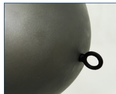
Bow tow-eye for quick link to DPD
