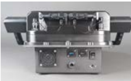
RNAV3 Casing mounted on custom desktop interface with all external ports required to support dive simulation
