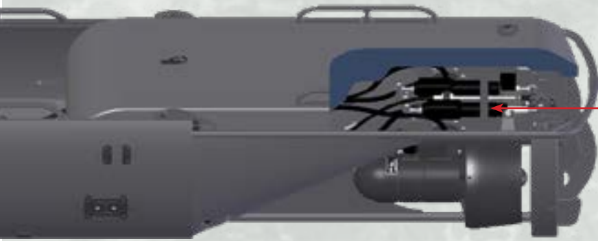
exposing installed RNAV3 and AP3 actuators
