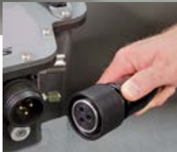
Jak-Lok Connectors installed on DPD3 Propulsion Battery
