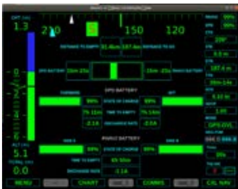
RNAV3 display of DPD3 Battery (fore/aft) operational parameters
