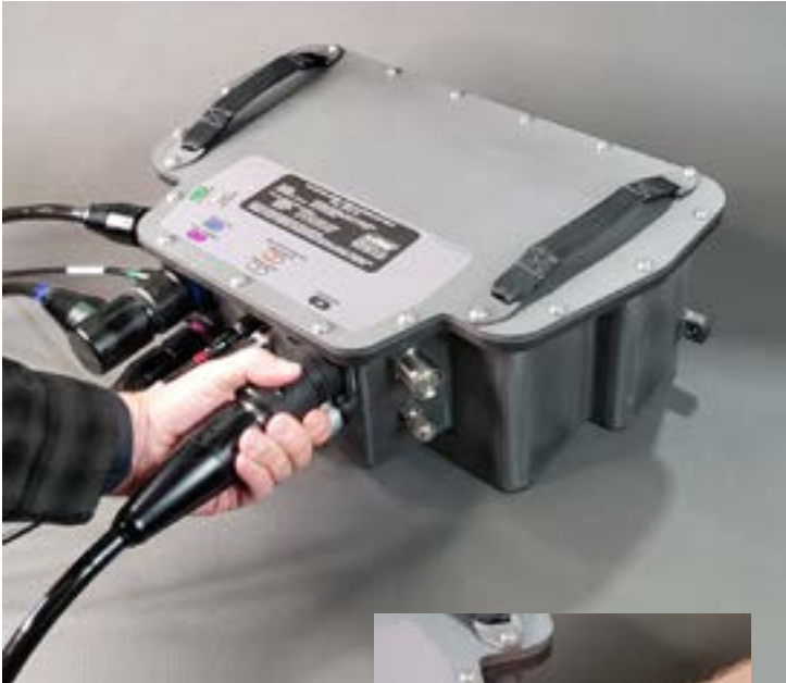
Jak-Lok Connectors installed on DPD3 Propulsion Battery
