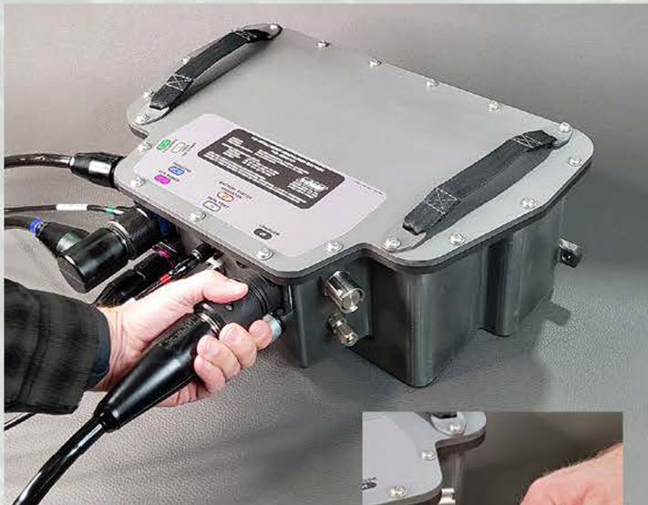
Jak-Lok Connectors installed on DPD3 Propulsion Battery
