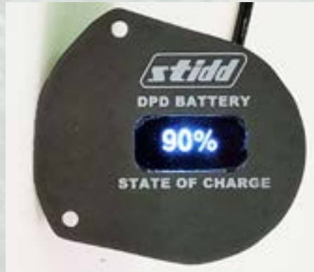
RNAV3 Battery Status Indicator (BSI) indicating 90% SOC.
