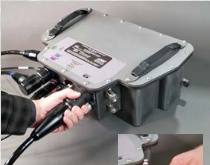
Jak-Loc Connectors installed on DPD3 Propulsion Battery
