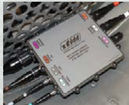
RNAV3 Battery Status Indicator (BSI) indicating 90% SOC.
